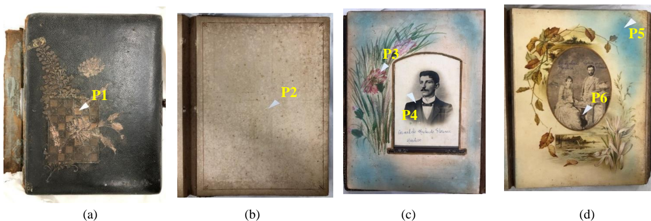
Figure 1: Locations of the measurement points in the photo album (a) P1 – album front cover; (b) P2 – endpaper; (c) P3 - rose flower engraving, P4 – photograph detail; (d) P5 – blue color, P6 – photograph detail.
