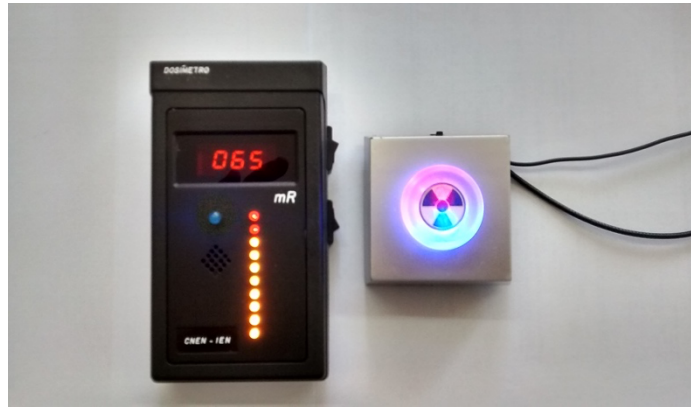
Figure 1: Devices developed to simulate a source and a radiation monitor.
