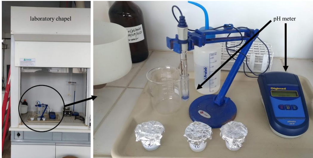
Figure 1: On the left, a fume hood with the equipment used in the assays. On the right, the pH meter and its probe.
