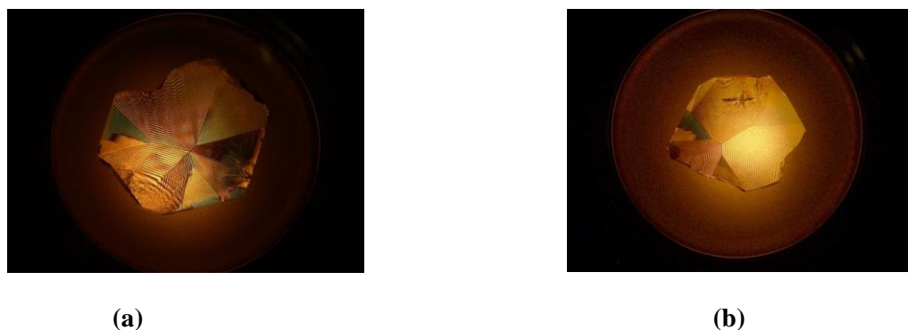
Figure 2: Images obtained in the polariscope in quartz plates of the Ametista do Sul (a) and (b) with Brazil Law twinning.
