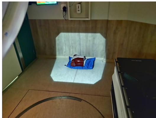
Figure 3: The Alderson phantom in the room floor treatment
