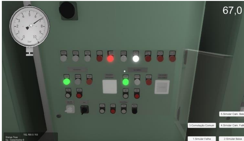
Figure 2: Electrical panel of oil pumps and malfunction menu.
